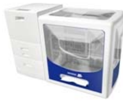
Figure 8. The Espresso print-on-demand machine, printing and binding books from a digital template.
